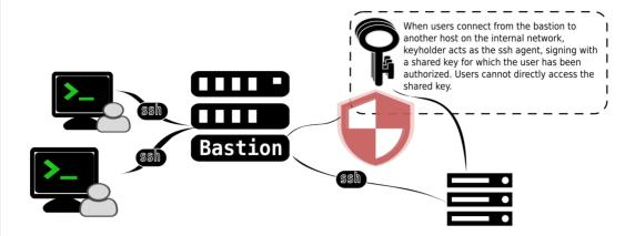
Keyholder, a newly open-sourced project from the Wikimedia Foundation, is a bit like that everwatchful security minion. For us, it allows authorized developers to access remote servers using an ssh key, to which it is the only user that has access. More specifically, Keyholder is an ssh-agent proxy that allows a group of trusted users to share an SSH identity without exposing the contents of that identity's private key.
